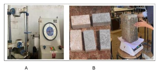
Fig.4 showing the tests of the brick Compression Strength Test (B) Water absorption Test
